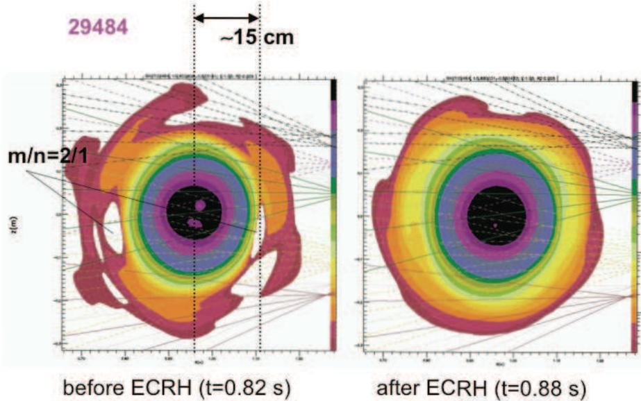
**Fig.2:** Localization of MHD islands from soft x-ray horizontal camera tomography in discharge #29484 ( $P_{ECRH}=1.0$  MW,  $r_{dep}=15$  cm).
