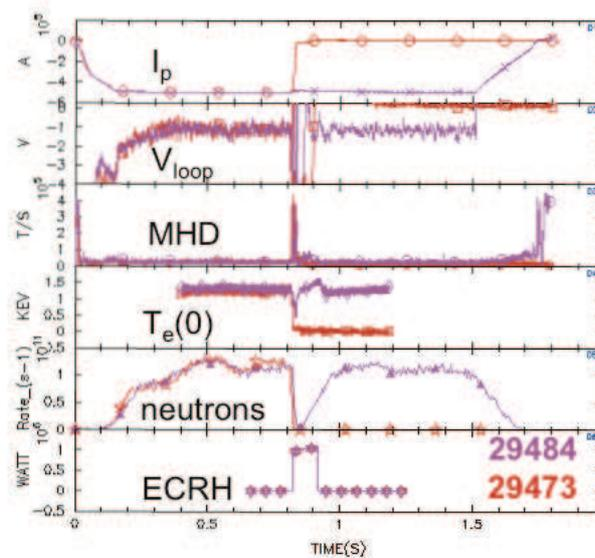
**Fig.1:** Disruption avoidance in Mo-injection discharges in FTU.
