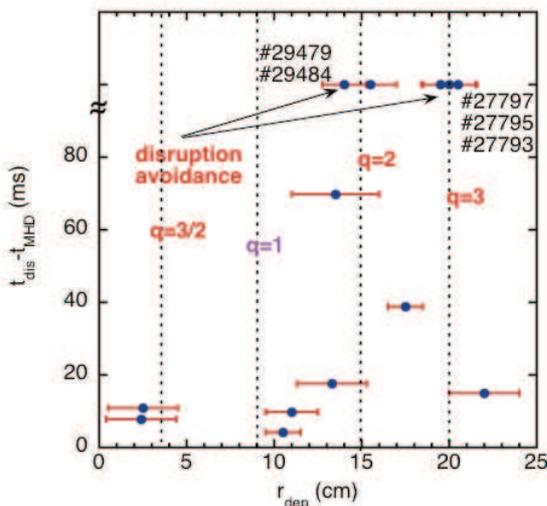
**Fig.3:**  $P_{ECRH}$  deposition scan:  $r_{dep}$  is evaluated using the ECWGB 3D quasi-optical ray-tracing code;  $t_{MHD}$  is the starting time of MHD activity and  $t_{dis}$  the disruption time.
