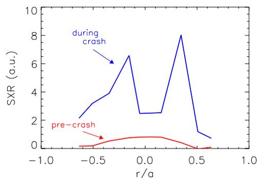
Fig. 5: Change in the radial profile of the SXR emission during a crash.
