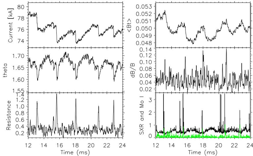
Fig. 1: Fluctuations in a typical discharge where  $\langle B_t \rangle$  is the average toroidal flux,  $dB/B$  is the total magnetic fluctuation level and in the last panel the SXR is in black and the MoI in green.
