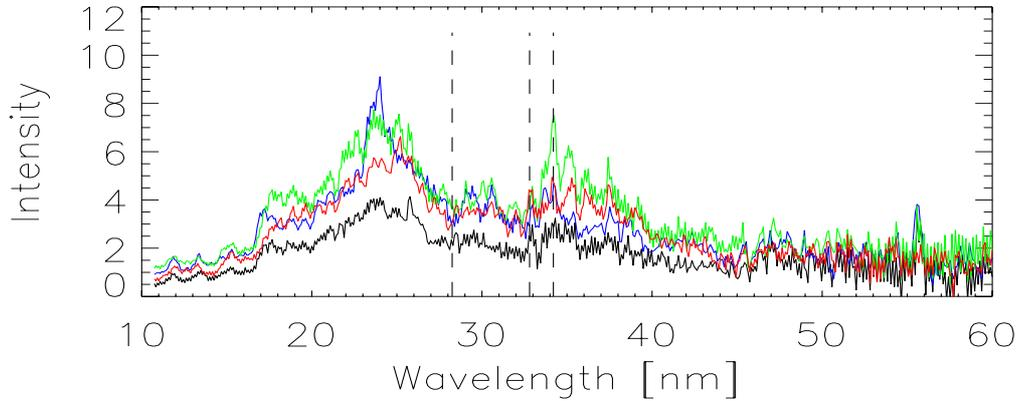
Fig 3: Time evolution of the VUV spectra from 10 to 60nm during the same crash event as in Fig. 2. The spectra are taken at 17.7ms (black), 17.9ms (blue), 18.2ms (green) and 18.4ms (red). Dashed lines show FeXV at 28.4nm, CrXIII at 32.8nm and MoXIII at 34.1nm.
