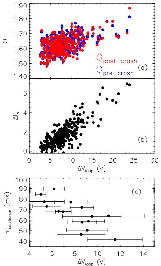
Fig. 4: Relationship between the step in loop voltage at the crash ( $\Delta V_{loop}$ ) and (a) pre- and post-crash  $\Theta$ ; (b) drop in  $I_p$ ; and (c) length of discharge.
