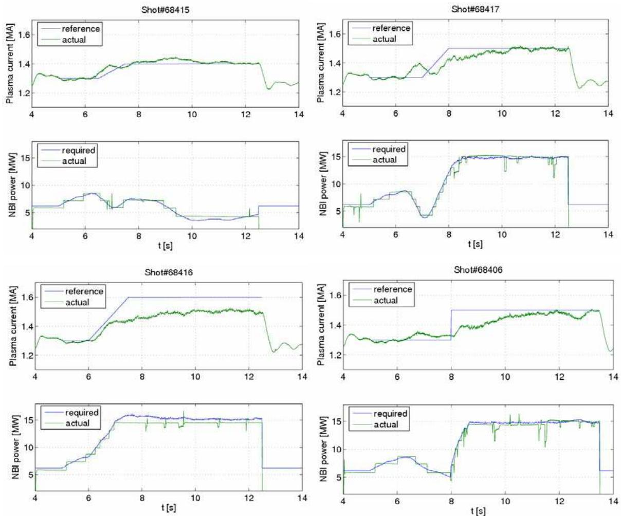
Figure 3. Examples of non-inductive plasma current control: plasma current (required and measured) and NBI power (requested and delivered) for shots# 68406, 68415, 68416, 68417.
