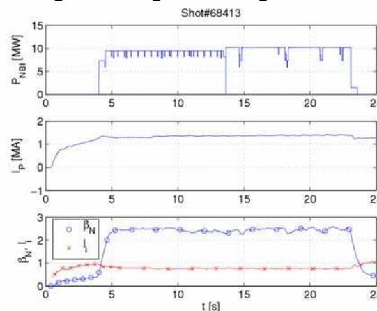
Figure 2. Time behaviour of plasma current, NBI power,  $\beta_N$  and  $I_i$
