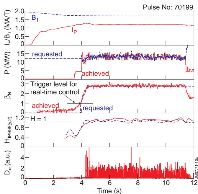
Figure 1. Time evolution of a typical high  $\beta_N$  pulse showing plasma current and magnetic field; requested and achieved NBI power; requested and achieved  $\beta_N$ ;  $H_{IPB98(y,2)}$ ; and  $D_\alpha$ , showing type I ELMs.  $H_{ITER98(y,2)}$  was evaluated using thermal stored energy from pressure profile integration (red) and  $W_{diamagnetic} - 1.5 \times W_{fast}$  using TRANSP NBI model [2] (blue).
