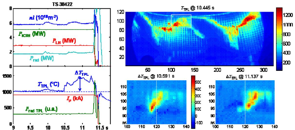
Fig. 3: left: time evolution of main discharge parameters with TPL surface temperature (from the box in the IR image on the right); right: IR image of a 30° sector of the TPL (axis in pixels) and  $\Delta T_{TPL} = T_{box}(t) - T_{box}(10.445 \text{ s})$  at 10.591 s and 11.137 s. Disruption occurs at 11.432 s. (TS-38422)
