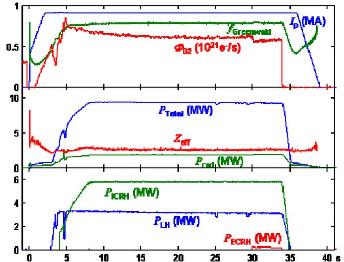
Fig. 1: time evolution of the main parameters of a 9.5 MW, 26 s discharge (TS-37685).
