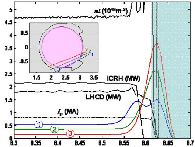
Fig. 2: Time evolution of main plasma parameters and three bolometer signals (u.a.) aiming at the Toroidal Pumped Limiter (TPL) region, before a disruption (TS-36687).
