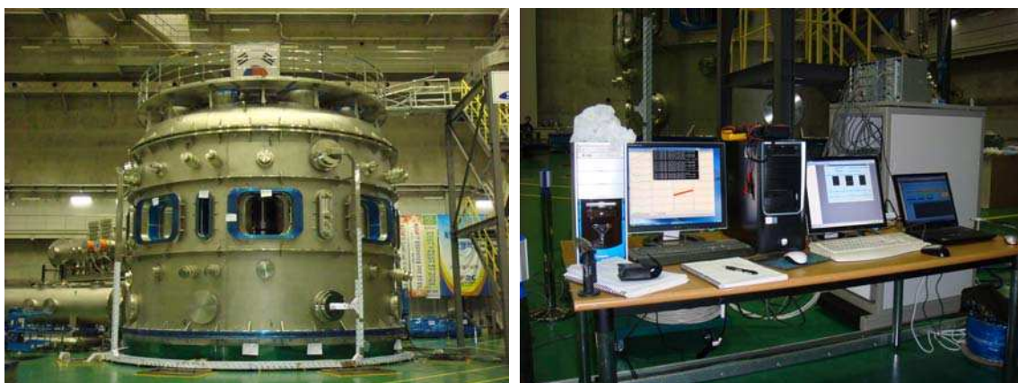
Fig. 2. The KSTAR tokamak and Rogowski coil calibration system.
