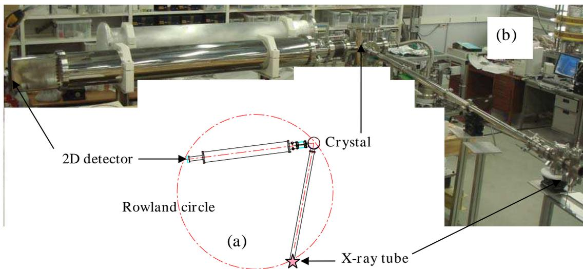
*Fig. 1. A design view (a) and fabricated XICS (b).*
