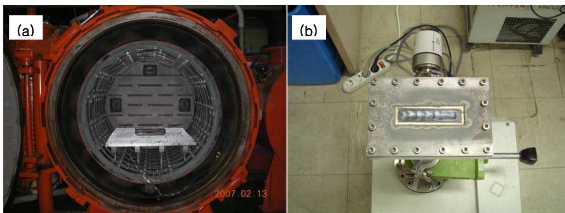
*Fig. 2. A vacuum brazing furnace (a) and sample piece of Be window (b).*
