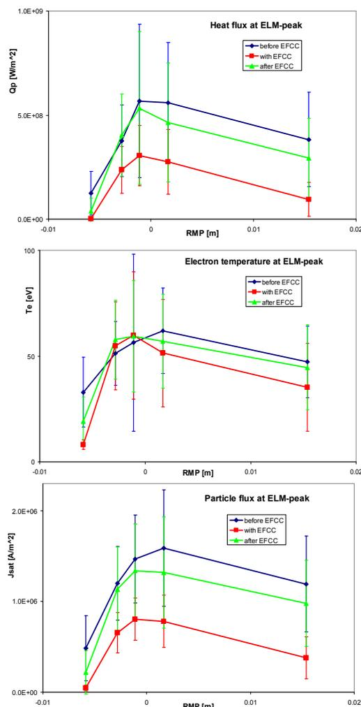
Fig. 7: Profiles at outer divertor during EFCC-experiments.
