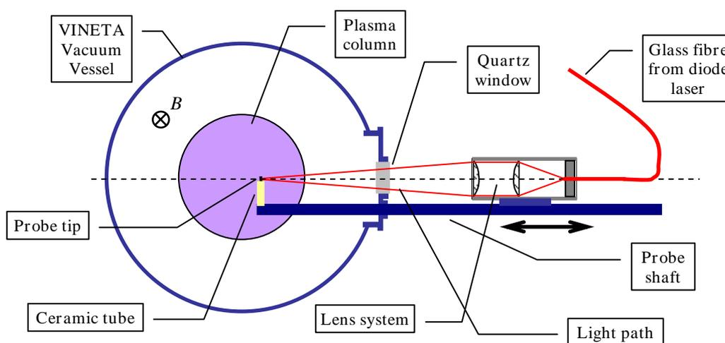
Fig. 1: Schematic of the radially moveable laser-heated emissive probe.
