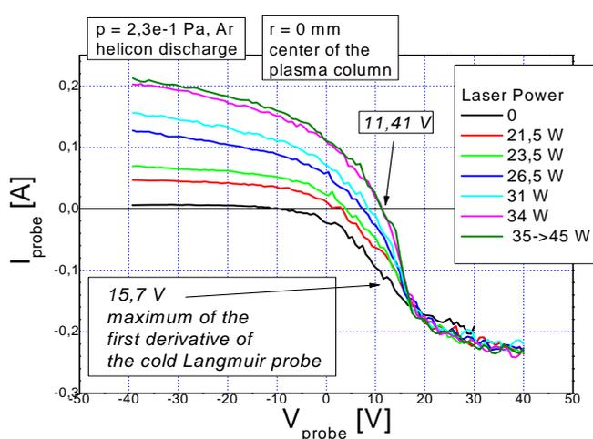
Fig. 2: Current-voltage characteristics of the laser-heated electron-emissive probe in the centre of the VINETA plasma column, showing its working principle. With increasing laser heating power the probe tip reaches sufficient emission so that its floating potential shifts towards the plasma potential. When the emissive probe is hot enough the floating potential is a good approximation of the plasma potential.
