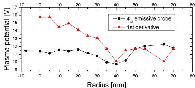
Fig. 3: Radial profiles of the plasma potential profile obtained with the laser-heated electron-emissive probe (black dots) and from the first derivative of the cold probe (red triangles) (left ordinate) and of the ion saturation current (blue asterisks) (right ordinate).
