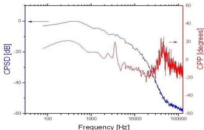
Fig. 4. Cross-power spectral density (CPSD) and corresponding cross-phase spectrum of the plasma and floating potential fluctuations.
