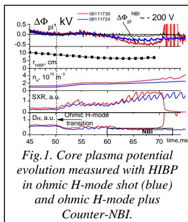
*Fig.1. Core plasma potential evolution measured with HIBP in ohmic H-mode shot (blue) and ohmic H-mode plus Counter-NBI.*
