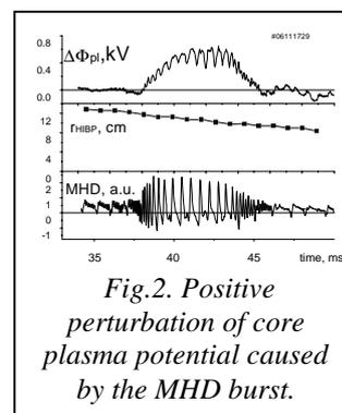
Fig.2. Positive perturbation of core plasma potential caused by the MHD burst.
