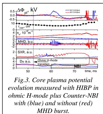
Fig.3. Core plasma potential evolution measured with HIBP in ohmic H-mode plus Counter-NBI with (blue) and without (red) MHD burst.
