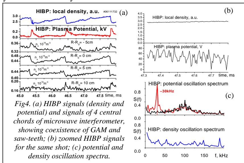
Fig.4. (a) HIBP signals (density and potential) and signals of 4 central chords of microwave interferometer, showing coexistence of GAM and saw-teeth; (b) zoomed HIBP signals for the same shot; (c) potential and density oscillation spectra.
