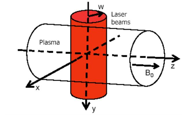
Figure 2. Plasma and scattering electromagnetic waves geometry (example for small angle forward scattering).
