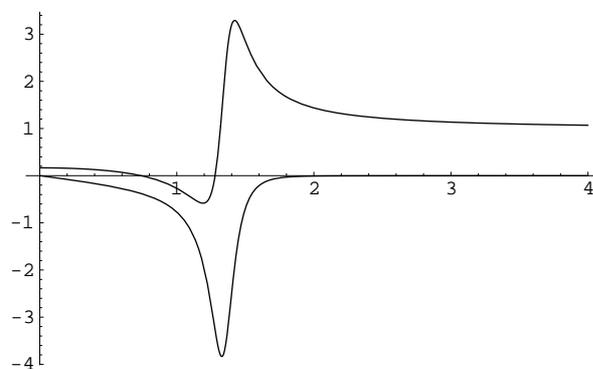
Figure 1 The ion structure factor  $\delta n$  as a function of the velocity  $v_{//}/c_s$ , for small  $k_{//} \lambda_D$ .
