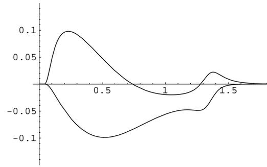
Figure 4. The structure factor as further weighed by the time-of-flight term, as a function of  $v_{\parallel}$
