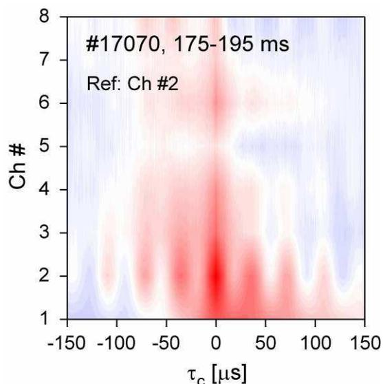
Fig. 4 Multi-channel, cross-correlation of BES signals with ch. 2 as reference from an ELMy H-phase of a discharge with 1.3 MW NBI power.
