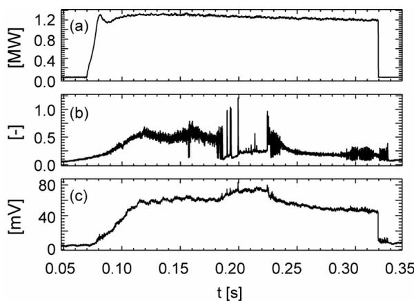
Fig. 1 Evolution of (a) SW NBI power, (b)  $D_\alpha$  intensity and (c) beam emission intensity from ch. #3 during discharge #17068 exhibiting L- and H-mode phases.
