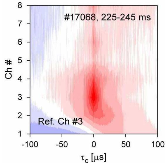
Fig. 3 Multi-channel, cross-correlation of BES signals from an L-mode phase of the discharge shown in Fig. 1.
