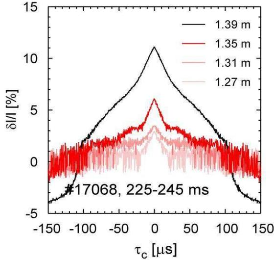
Fig. 2 Square root of the auto-covariance of BES signals normalized with the signal level from chs. #2-5 during an L-mode phase of the discharge shown in Fig. 1.
