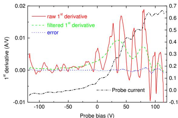
Figure 3: 1<sup>st</sup> derivatives: raw (solid) and after filtering (dash), guessed error (dot), and current (dash-dot).
