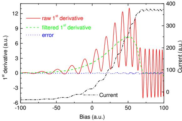
Figure 1: 1<sup>st</sup> derivatives: raw (solid) and after filtering (dash), guessed error (dot), and  $I(V)$  data (dash-dot) used in the model test.
