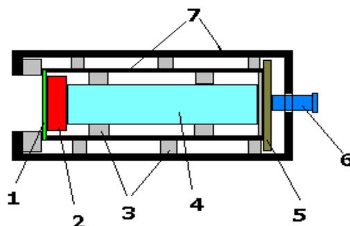
**Fig. 1.** Schema of piezodetector: 1 - protective insulator, 2 - piezo-ceramic pill, 3 and 5 - elastic gaskets, 4 - lead rod, 6 - hold-down screw, 7 - metal case (screen)
