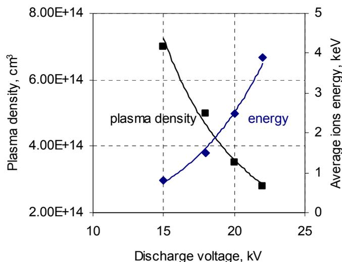
**Fig. 2.** Influence of the discharge voltage on the plasma density and the average ions energy
