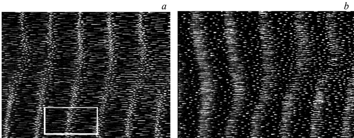
Fig. 1. Video frame of the excited nonlinear dusty-acoustic wave in fixed co-ordinates (a) and moving co-ordinates (b).
