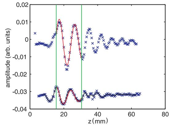
Figure 5: Interferometric traces in a dust-free (top trace) and dusty (bottom trace; vertically shifted) argon discharge.
