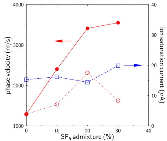
Figure 3: Full circles: phase velocity of the ion acoustic wave as function of the SF<sub>6</sub> admixture. Open circles: phase velocity corrected for increase in electron temperature. Squares: ion saturation current of a plane probe.
