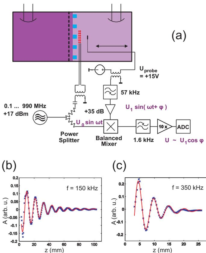
Figure 1: (a) Double plasma device with r.f. interferometer, (b) interferometric trace and fit function in pure argon gas at 150 kHz, (c) same at 350 kHz.
