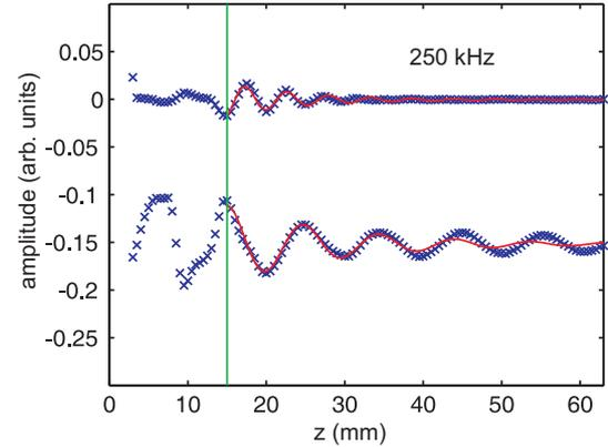
Figure 2: Interferometric wave signal in pure argon (top trace) and Ar-SF<sub>6</sub> mixture (bottom trace; vertically shifted). ( $n_e = 5 \times 10^{15} \text{ m}^{-3}$ ,  $T_e = 2 \text{ eV}$ )
