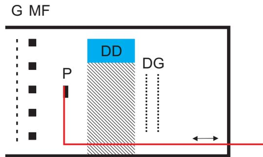
Figure 4: Dust is released from a dispenser (DD) with 95 mm diameter and fills the hatched region between the double grid exciter (DG) and the moveable probe (P).
