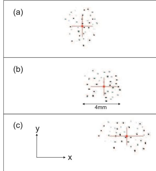
Figure 2: Sloshing and stretching of the dust cloud at low modulation frequency  $f_{mod} = 4$  Hz. ( $U_a = 70$  V,  $U_{mod} = 10$  V<sub>pp</sub>). (a) left turning point, (b) equilibrium position, (c) right turning point.
