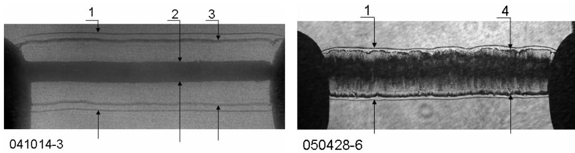
Fig. 1. Optical images of the discharge channel upon exploding a) tungsten ( $t = 590$  ns) and b) copper ( $t = 415$  ns) wires in air ( $U_0 = 20$  kV,  $l = 12$  mm,  $d = 25$   $\mu$ m).
