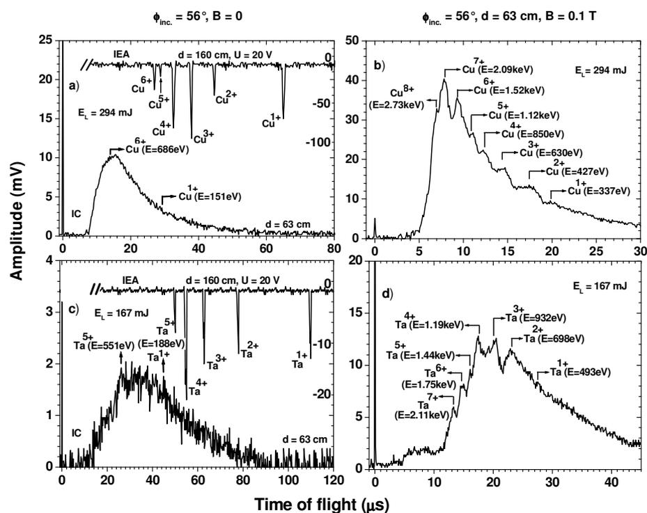
Fig. 2: TOF spectra comparison for Cu (a, b) and Ta (c, d) without and with magnetic field.
