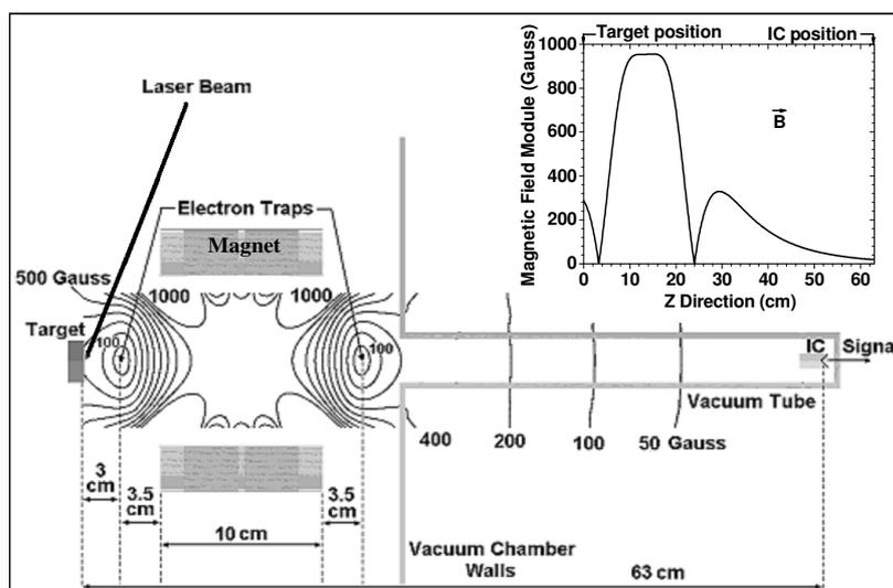
Fig. 1: Scheme of the experimental set-up and module of magnetic field (inset).
