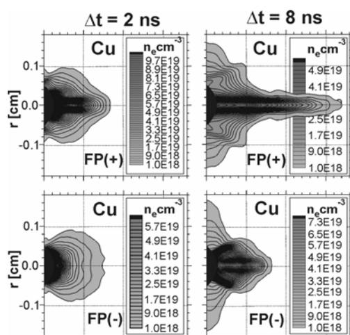
Fig.3. Sequences of electron isodensitograms for Cu target and different laser focus positions FP.  $E_L=(69\pm 2)\text{J}$ ,  $d_L=500\mu\text{m}$ .
