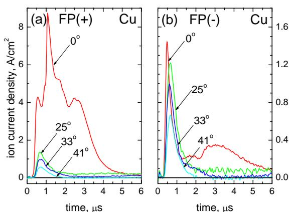
Fig.1. Ion collector signals from Cu target for different laser focus positions FP.  $E_L=(69\pm 2)\text{J}$ ,  $d_L=500\mu\text{m}$ ,  $L_{IC}=50\text{cm}$ .
