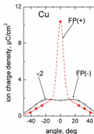
Fig.2. Angular distributions of the ion charge density for ions of velocities in the range  $(0.2-2)\times 10^8\text{cm/s}$ .  $E_L=(69\pm 2)\text{J}$ ,  $d_L=500\mu\text{m}$ ,  $L_{IC}=50\text{cm}$ .
