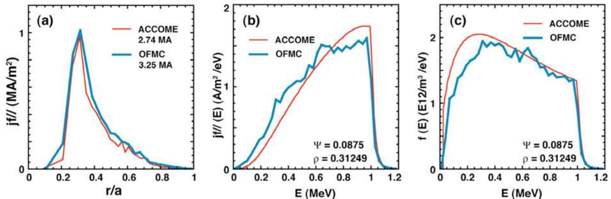
Fig.4 (a) The fast ion current density ( $j_{FI}$ ). (b) The contribution to  $j_{FI}$  and (c) the fast ion distribution function in the energy space.
