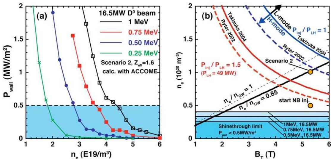
Fig.1 (a) Electron density dependence of the shinethrough heat load on the far wall ( $P_{wall}$ ) for 16.5 MW  $D^0$  beam injection to Ref. Scenario 2 at 0.25, 0.5, 0.75 and 1 MeV. (b) DT operation space defined by the shinethrough limit, density limit and L-H transition boundary, where the total injection power ( $P_{inj}$ ) is 73MW and  $q_{05}=3$ .
