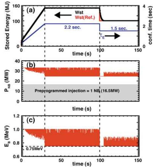
Fig.3 Simulation of the plasma stored energy ( $W_{ST}$ ) FB control. (a) Reference (black) and calculated (red)  $W_{ST}$  and energy confinement time ( $\tau_E$ ). (b) Total NB power. (c) FB controlled beam energy.
