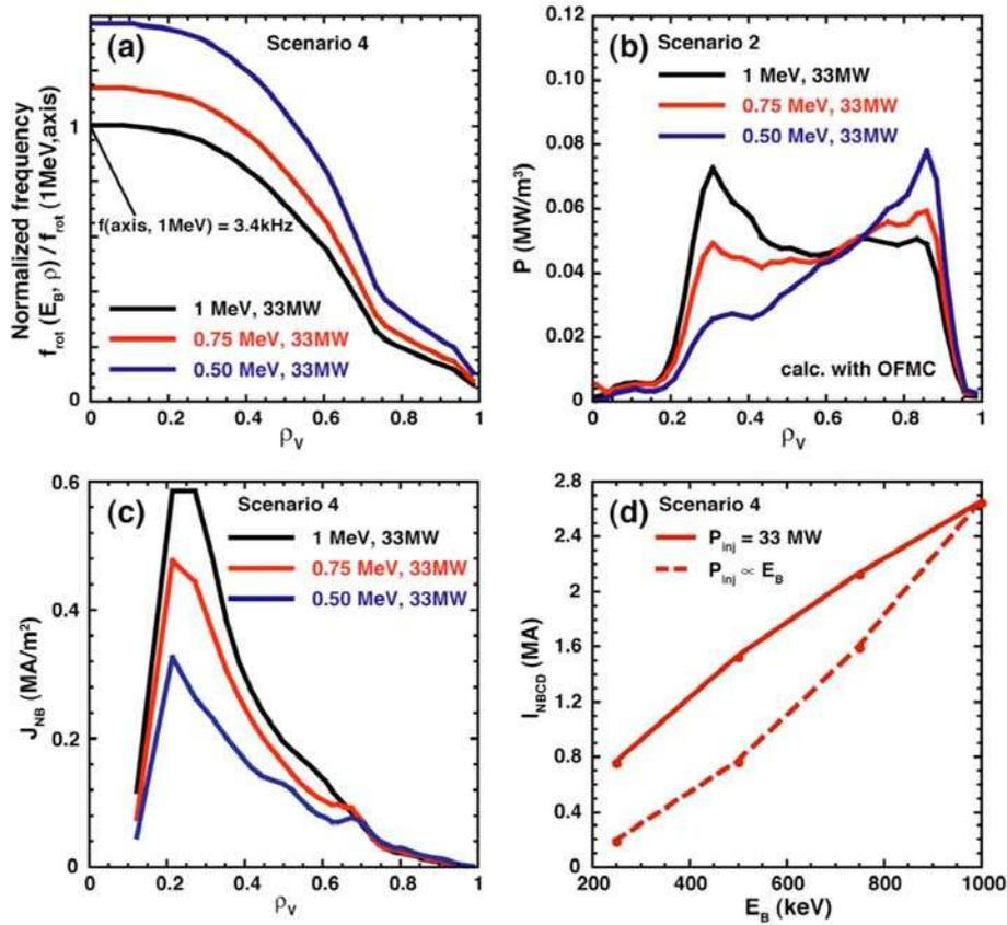
Fig.2 (a) Toroidal rotation frequency profiles for Ref. Scenario 4, (b) heating profiles for Ref. Scenario 2 and (c) NBCD profiles by 2 NBIs (33MW) at 0.5, 0.75 and 1 MeV. (d) Beam energy dependences of the total NBCD for Ref. Scenario 4 by the 33MW constant  $P_{inj}$  (solid) and the beam energy proportional  $P_{inj}$  (dashed).
