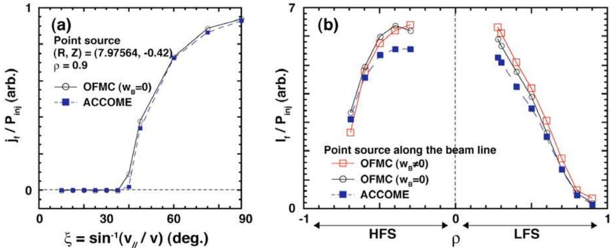
Fig.5 ACCOME - OFMC comparisons. (a) Pitch angle ( $\xi$ ) dependence of the NBCD for the given point source of the fast ions at  $(R, Z)=(7.96, -0.42)$ , where the finite banana width effect turned off in OFMC. (b) NBCD for point sources along the NB trajectory.
