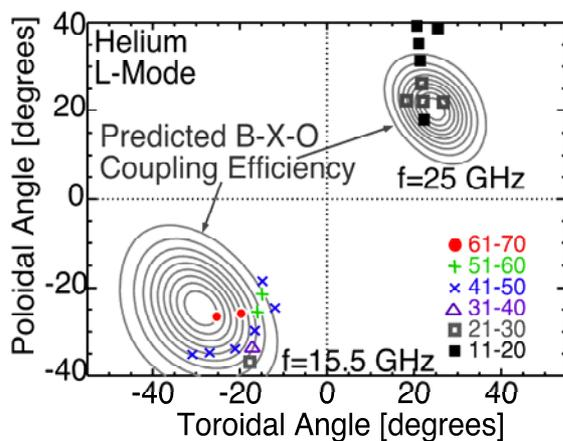
Fig. 5. Conversion efficiency at 15.5 and 25 GHz: grey contours, predicted; colored symbols, measured in L-mode plasmas
