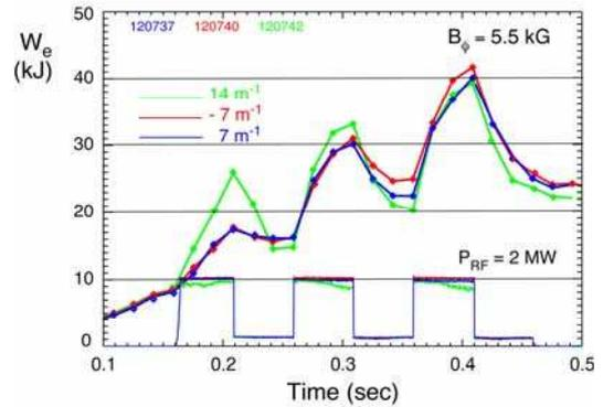
Fig. 2. Electron stored energy versus time and  $k_{//}$  at  $B_T = 5.5 \text{ kG}$ .
