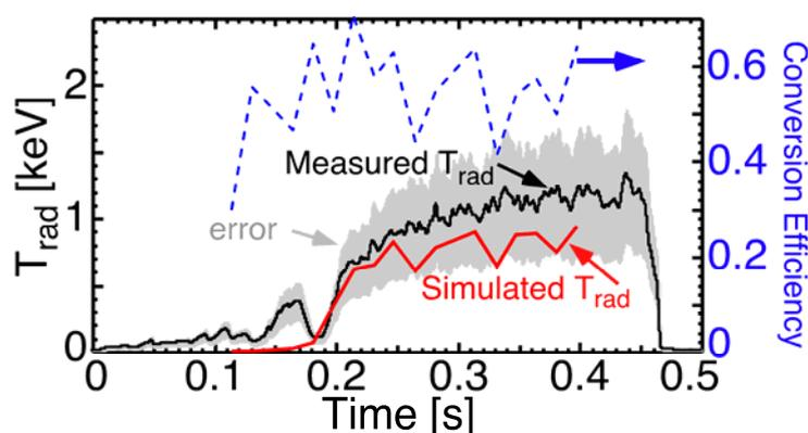
Fig. 6: EBW  $T_{rad}$ : black, measured; red, simulated. Simulated conversion efficiency, dashed blue.
