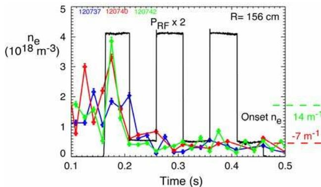
Fig. 3. Edge electron density (2 cm in front of Faraday shield) against time corresponding to curves in Fig 1.
