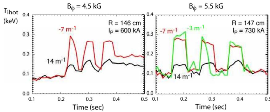
Fig 4. Edge ion heating as a measure of PDI losses. (Helium)
