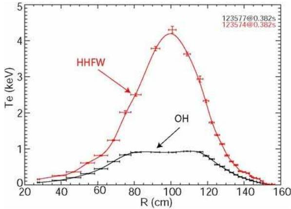
Fig. 1. Overlay of  $T_e(R)$  for plasma with 1.8-MW HHFW at  $k_{//} = -7 \text{ m}^{-1}$  and ohmic reference discharge at  $t=0.382 \text{ s}$ .
