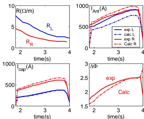
Figure 4 Evolution of the antenna loading resistances for a discharge where the plasma is slowly shifted 4 cm away from the antenna. Currents measured at the antenna and at the capacitor and phase difference between the currents in the left (L) and right (R) straps. The measured values of the currents (plain lines) are in good agreement with the values deduced from the transmission line model associated with the measurements in the transmission lines (dashed lines).
