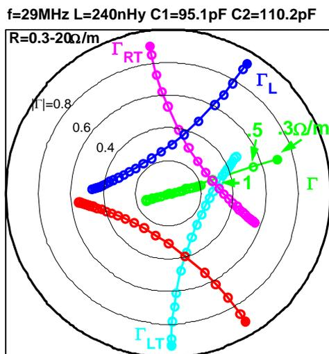
Figure 3 Reflection coefficients at the feeding points of the two straps of the CT antenna ( $\Gamma_L$  and  $\Gamma_R$ ), at the T-junction in the two branches of the CT ( $\Gamma_{LT}$  and  $\Gamma_{RT}$ ) and after the T-junction ( $\Gamma$ ) in the Smith's chart for  $R_A$  varying between  $0.3\Omega/m$  and  $20\Omega/m$  (circles) Load resilience inside the  $|\Gamma|=0.2$  circle. Circles at  $|\Gamma|=0.4$ ,  $0.6$  and  $0.8$  are also shown.
