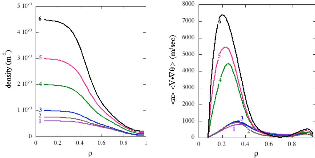
Figure 3 (left) – Model plasma density profiles used for moments method analysis of the LHD SDC regime, Figure 4 (right) – Predicted LHD poloidal flow velocity profiles obtained from the PENTA model.
