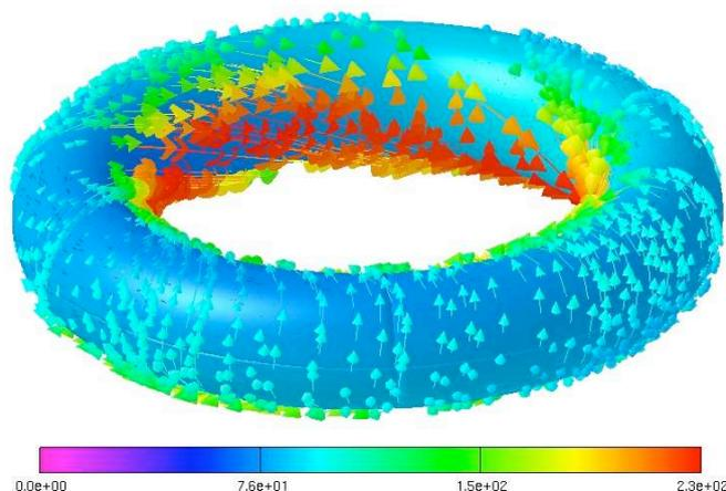
Figure 9 (left) – Ion flow velocity profiles for rippled tokamak, Figure 10 (right) – 3D arrow visualization of vector flow velocity field in rippled tokamak.
