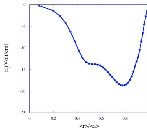
Figure 7 (left) – ITER equilibrium, showing rippled magnetic field strength, Figure 8 (right) – Ambipolar electric field profile for rippled tokamak.
