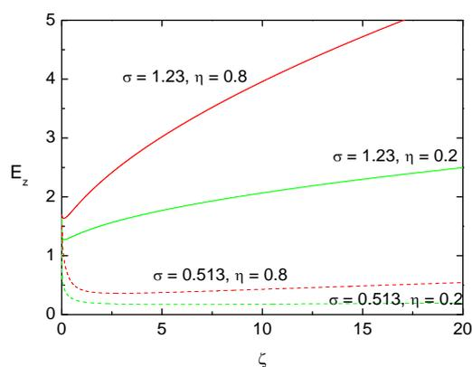
Fig. 5. Electric field z-component axial profiles at  $\gamma = 0.85$  and various plasma radii and metal rod thicknesses
