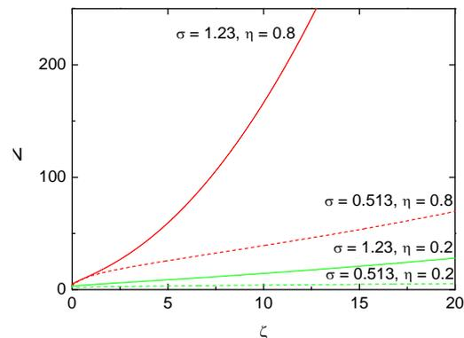
Fig. 4a. Plasma density axial profiles at  $\gamma = 0.85$  and various plasma radii and metal rod thicknesses
