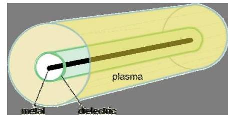
*Fig. 1. Coaxial discharge structure*
