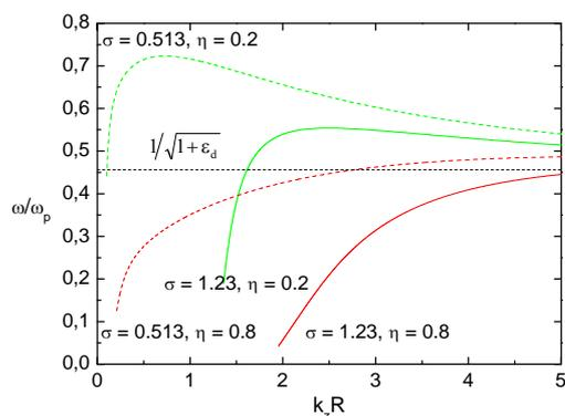
Fig. 4a. Phase diagrams at  $\gamma = 0.85$  and various plasma radii and metal rod thicknesses
