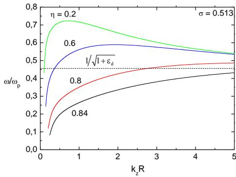
Fig. 2a. Phase diagrams at  $\sigma = 0.513$ ,  $\gamma = 0.85$  and various metal rod thicknesses
