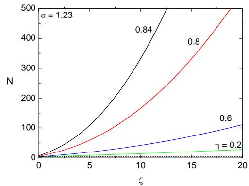
Fig. 3b. Plasma density axial profiles at  $\sigma = 1.23$ ,  $\gamma = 0.85$  and various metal rod thicknesses
