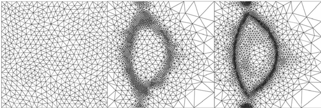
Figure 2: Sequence of meshes used in toroidal equilibrium calculation. Meshes are adapted to resistivity profile with 956(l), 3554(c), and 5512(r) elements.
