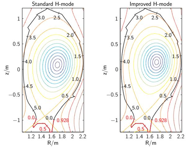
Figure 4: Comparison of magnetic geometry for the Standard and Improved H-mode pulses # 17216 and # 17219, respectively.
