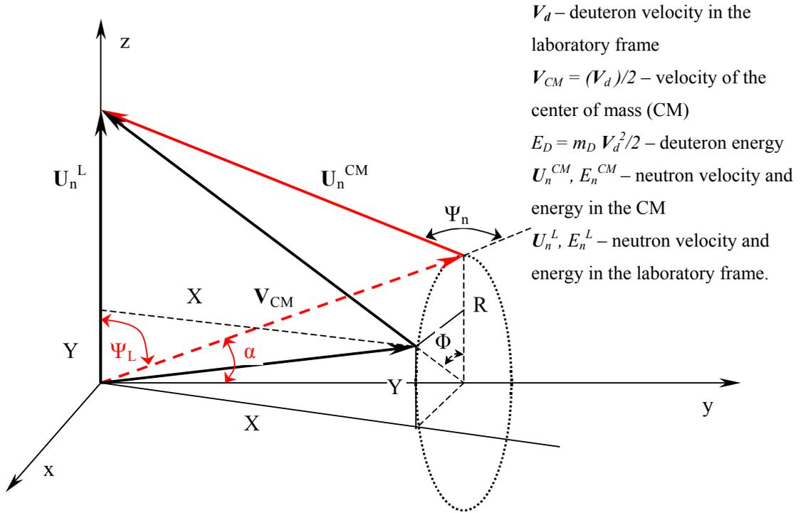
Fig.1. Vectors diagrams for deuteron fusion collisions
