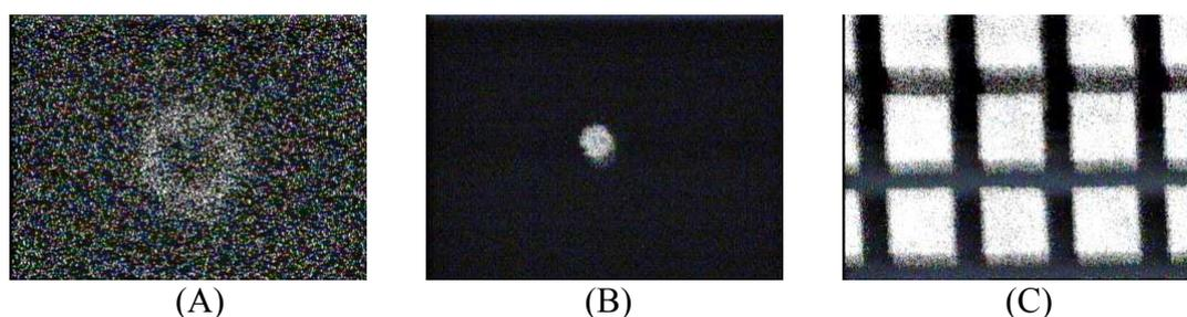
Fig. 2. Exemplary images obtained with different X-ray sources: (A) - with the lamp of a cold cathode Dina 1, (B) and (C) - with laser-plasma source.
