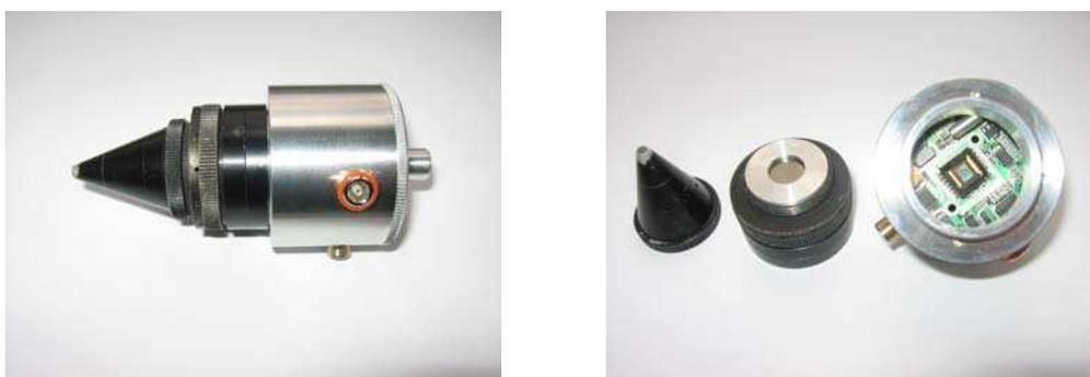
Fig. 1. Overall view and internal structure of the CCD pinhole camera.
