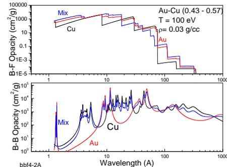
Fig. 4 Bound-Free and Bound-bound opacity of the plasma at a temperature of 100eV and plasma density of 0.03g/cc for copper (—), gold (—) and Au-Cu (—) Mixed targets.
