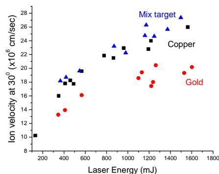
Fig. 5. Ion velocity as a function of laser energy for copper (■), Gold (●) and Au-Cu Mix (▲) targets.
