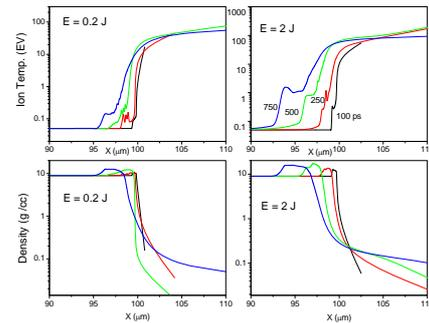
Fig.3: Spatial profiles of ion temperature and density for laser energy 0.2 Joule and 2 Joules.
