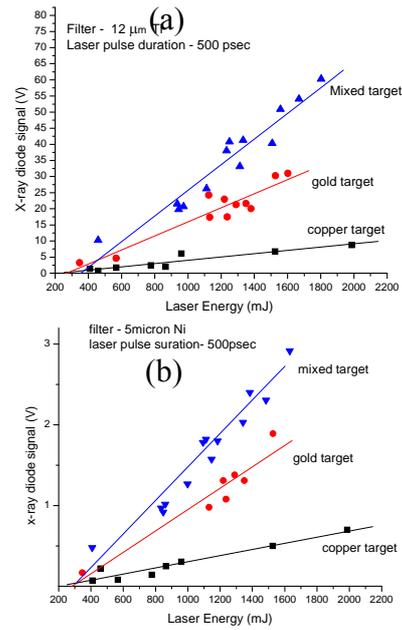
Fig. 2. –X -ray emission as a function of Laser energy for the two pin diodes.(a)-Nickel filter (b)-Titanium filter
