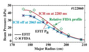
FIG. 3. Comparison of beam-ion pressure profiles and relative FIDA profile. The FIDA signal is averaged over E<sub>2</sub> between 40 keV and 80 keV.
