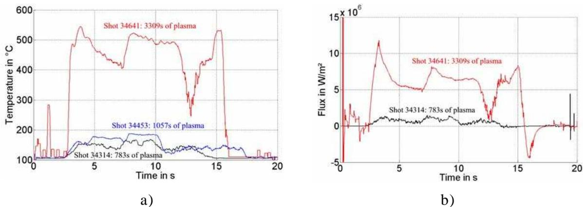
Figure 1a: Temperature evolution of three similar shots at three dates
