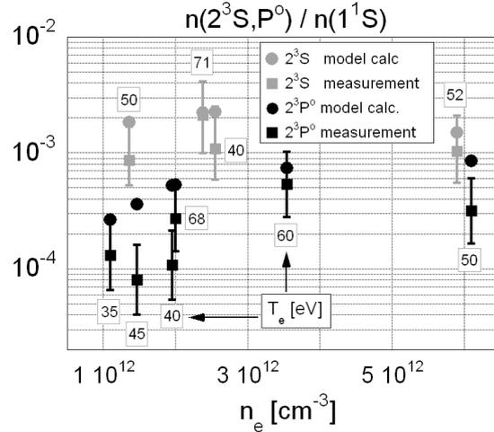
FIGURE 1. Calculated and measured relative populations of the levels  $2^3S$  and  $2^3P^o$ .
