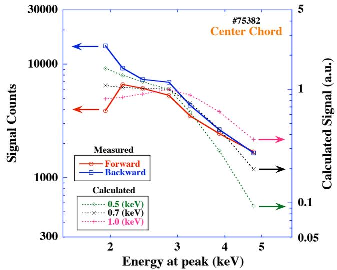
Figure 4: Signal intensity near the center chord plotted against the photon energy at the maximum efficiency for each filter combination. The calculated intensities for the electron temperatures of 0.5, 0.7 and 1.0 keV are also plotted.
