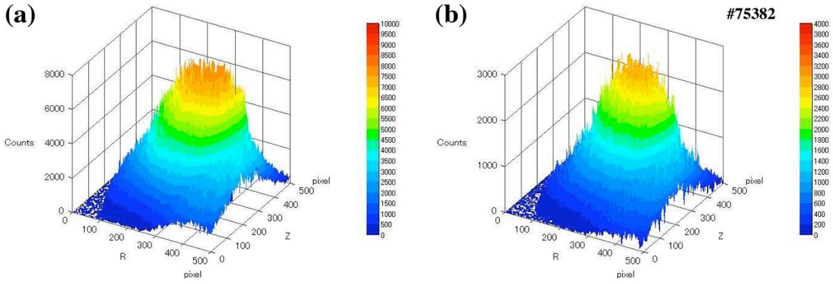
Figure 3: Contours of the two dimensional images obtained from the signal differences (a) between 70 and 100  $\mu\text{m}$  filter thicknesses, and (b) between 450 and 850  $\mu\text{m}$ .
