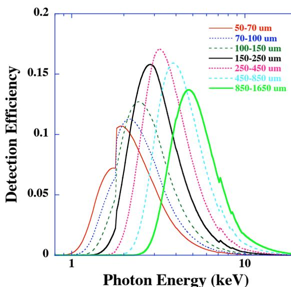
Figure 2: Detection efficiency curves for the differences between adjacent Be filter thicknesses used in this study, including the CCD quantum efficiency.
