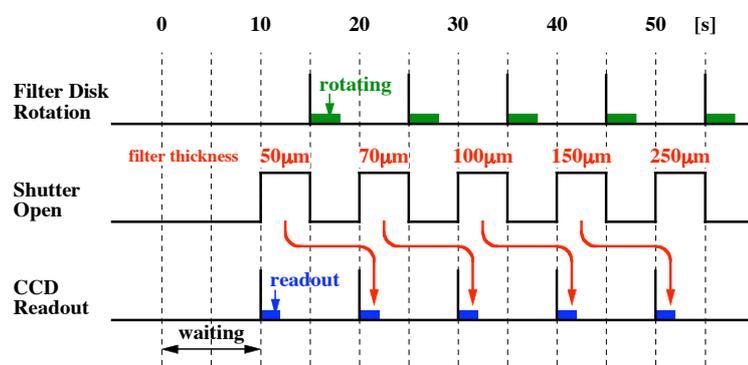
Figure 1: Timing chart of the filter disk rotation, the shutter open, and the CCD readout.
