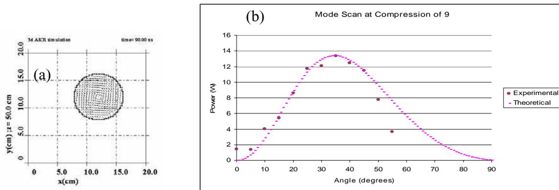
Figure 4: (a) 3D simulations in KARAT of the 4.45GHz mode structure of the apparatus and (b) the antenna pattern measured from the experiment
