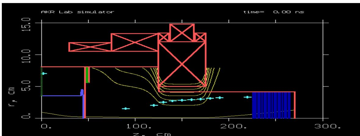
Figure 2: KARAT representation of the geometry in 2D showing electron accelerator, magnetic field solenoids and flux lines
