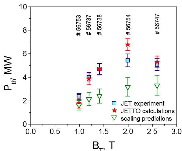
Fig.2 Comparison of the L-H power threshold computed with the JETTO code to the values obtained in experiment and predicted by the inter-machine scaling, for the set of discharges with various magnetic field.
