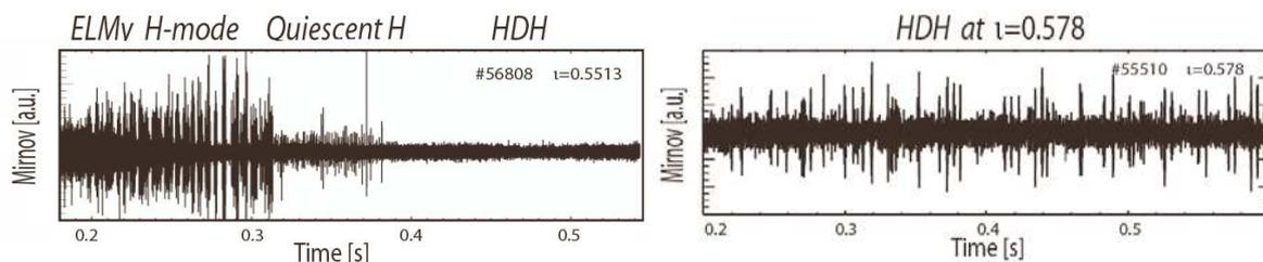
Figure 3. Micro-ELM activity in the two usually ELM-free H-modes of W7-AS in the raw Mirnov signals.
