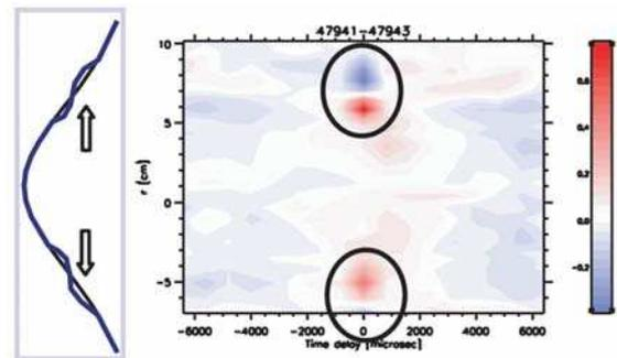
Figure 1. Appearance of ELM-like transients in the cross-correlation function of the ECE diagnostic. With pattern-recognition technique the profile flattening is detected and shown in Figure 2.
