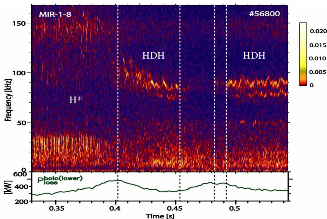
Figure 4. Spectrogram of the Mirnov diagnostics and time evolution of the impurity radiation for the Quiescent H mode and two HDH mode phases.
