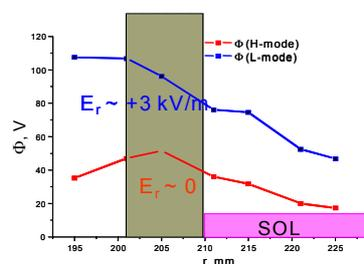
Fig. 6 Floating potential profiles measured in Ohmic L- and H-modes with Langmuire probes
