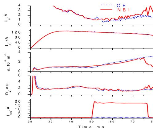
Fig.2 Evolution of loop voltage  $U_p$ , plasma current  $I_p$ , average density  $n$ ,  $D_\alpha$  intensity and NBI emission current  $I_{NBI}$  in Ohmic H-mode (dotted) in comparison with counter-NBI regime (solid)
