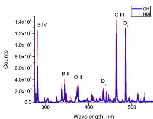
Fig.1 Plasma emission spectra in Ohmic H-mode in comparison with counter-NBI regime
