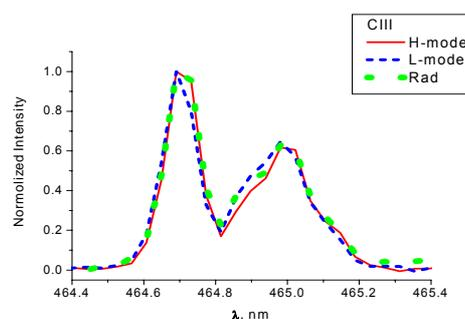
Fig.4 C III spectra in Ohmic H- and L-modes measured in toroidal direction in comparison with reference (non shifted) spectrum measured along the major radius (Rad)
