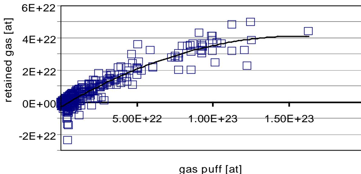
Fig.4: Retained amount of gas versus gas puffed during the divertor phase for the discharges 19990-20580.
