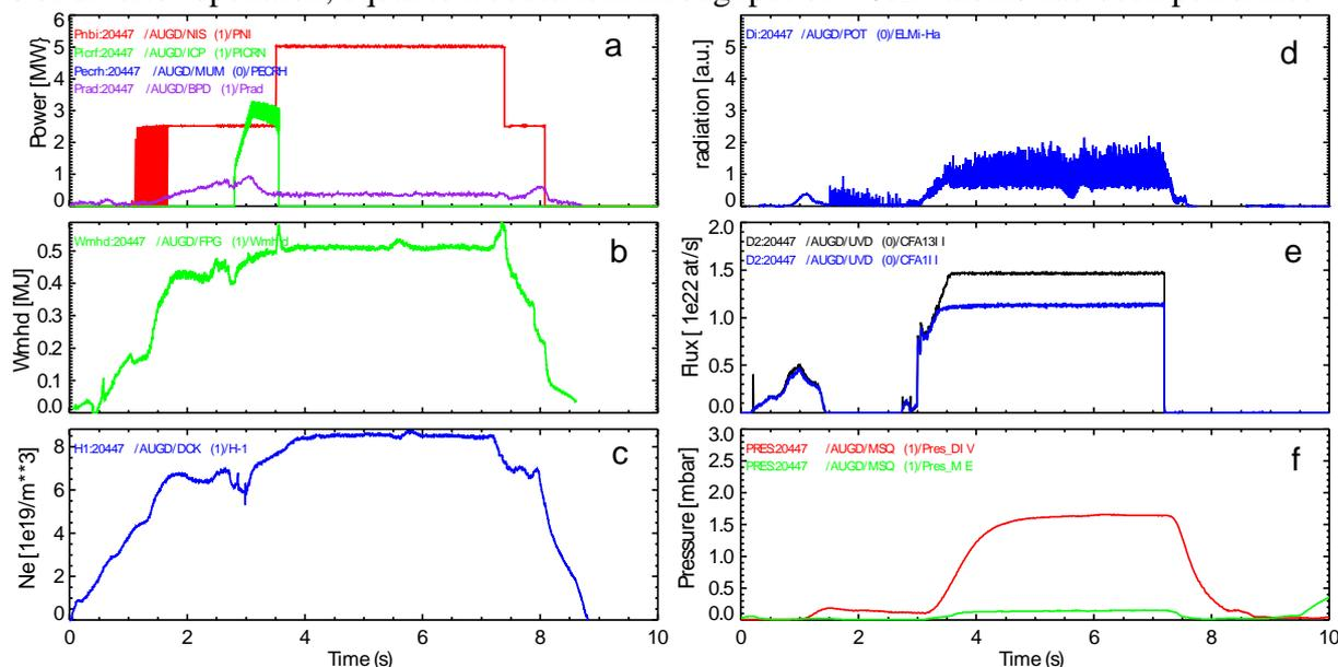
Fig.1: Main parameters of the plasma discharge 20447, showing time traces of the heating and radiation powers (a), energy content (b), line-averaged density (c), ELM behaviour (d), gas puffing rates (e) and divertor pressure (f)
