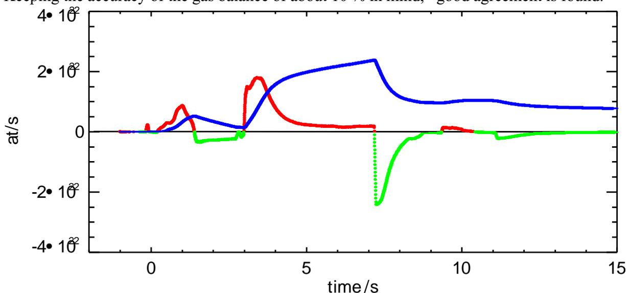
Fig.3: Total gas balance for shot 20447. Phases of gas deposited in the vessel are indicated in red, phases of vessel depletion in green. The integral is shown in blue.
