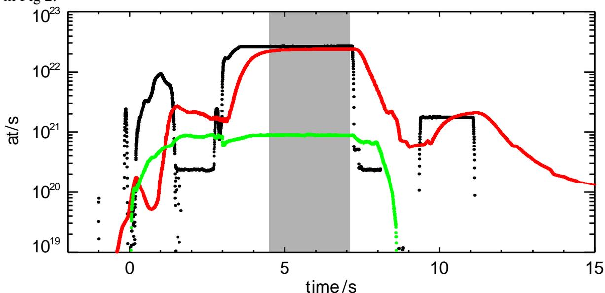
Fig.2: Time resolved gas rates for shot 20447. The rate of puffed gas is indicated in black, the pump rate in red and the plasma inventory in green. The “puff=pump” phase is indicated in grey.
