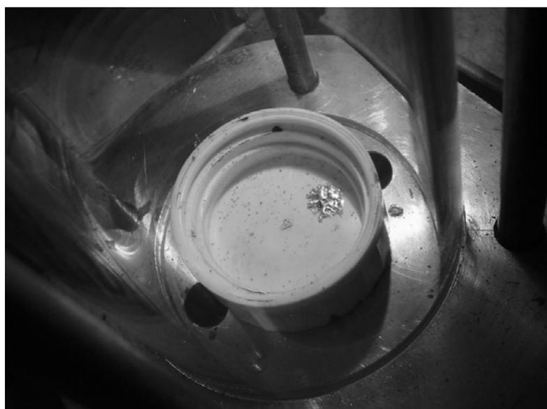
*Fig.3. Photo of the test-bed target hinted by a Li liquid jet.*
