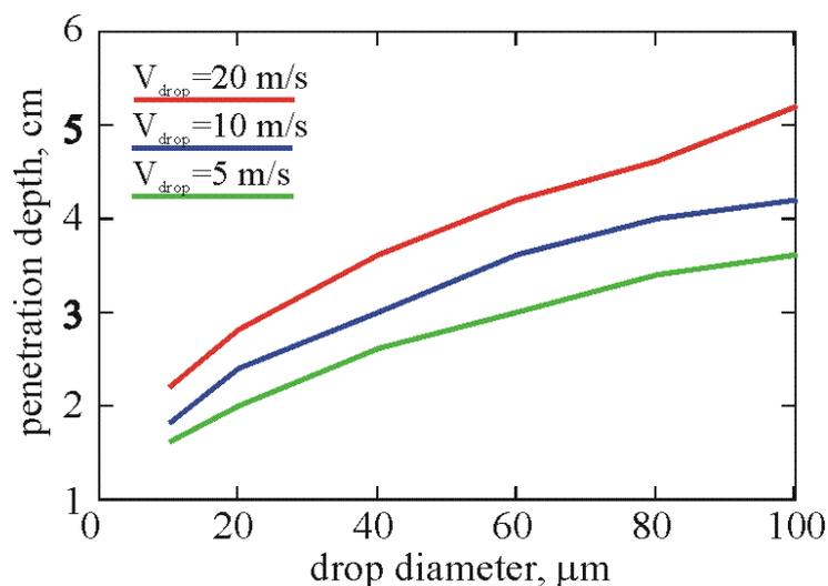
Fig.1. Simulated penetrations of Li droplets in T-10 plasma
