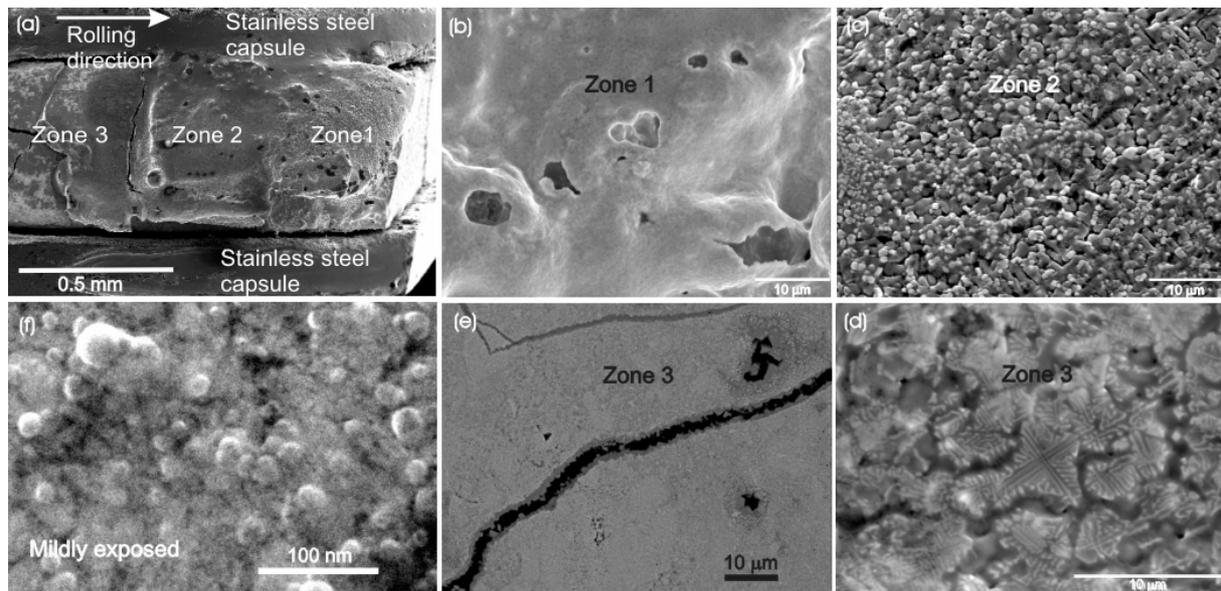
Figure 2 – (a) Surface of the rolled W-nDiamond exposed to the edge plasma (perpendicular to B). (b) Surface displaying evaporation. (c) Surface with carbide formation. (d) Surface displaying eutectic dendrites. (e) Cross-section showing molten stainless steel inside cracks. (f) Mildly exposed material exhibiting a dispersion of nDiamond particles.
