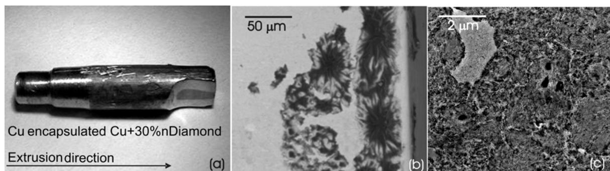
Figure 1 – (a) Extruded Cu-nDiamond sample exposed to the edge plasma. (b) Cross-section perpendicular to B showing craters. (c) Cross-section parallel to B immediately below the crater zone showing an extremely fine microstructure.
