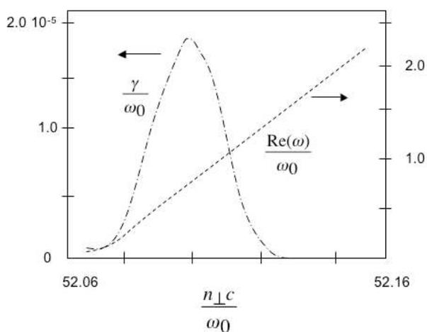
Figure 2. Solution of Eq. 1 for typical parameters of the FTU plasma periphery. For the low frequency driving mode, the frequency and growth rate (normalised to the pump frequency) are plotted vs. the normalised perpendicular wavenumber.
