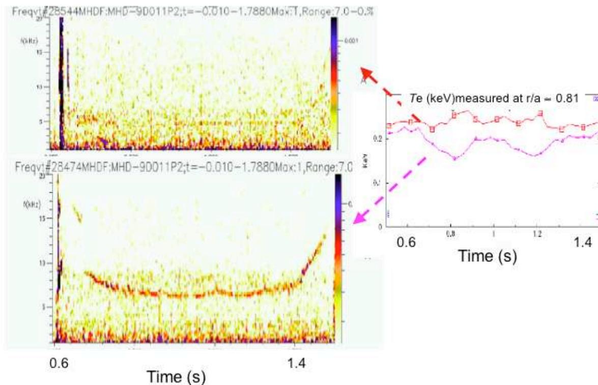
Figure 1. Comparison in similar shots of FTU performed with lithized (low recycling) and boronised vessel of the time evolution of the MHD spectrograms (Fig. 1 a) and the electron temperature at the plasma periphery (Fig. 1 b), considering the same time window.
