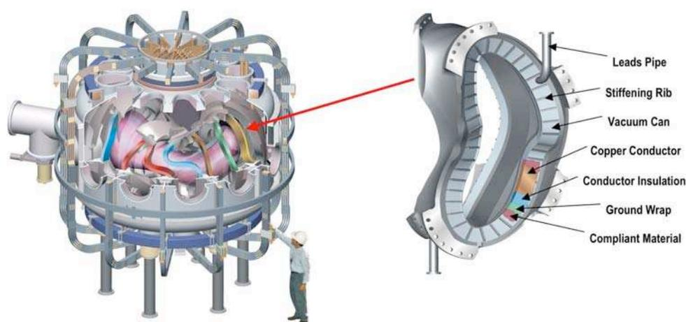
Fig. 2. Construction concept for QPS compact stellarator device.
