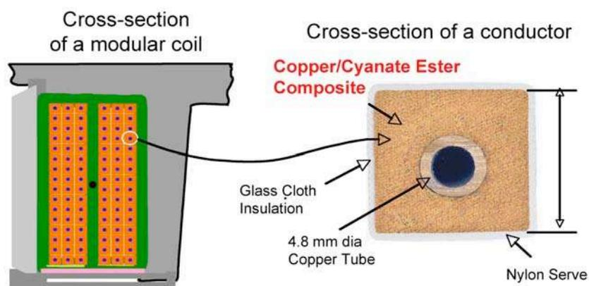
Fig. 4. Cross-sectional views of QPS winding and conductor.
