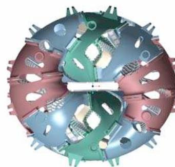
Fig. 3. QPS modular coil forms.
