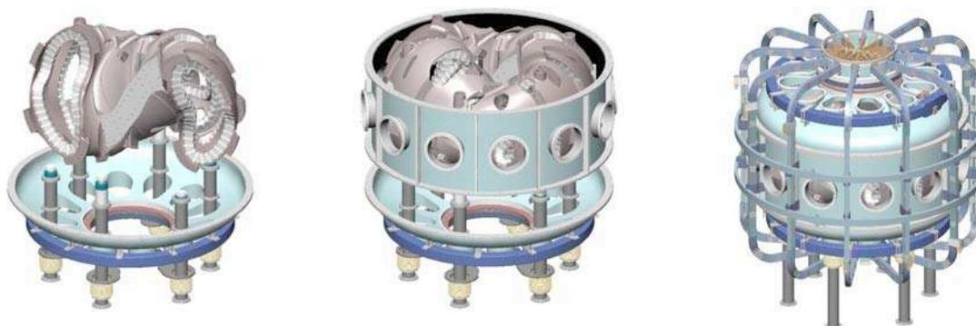
Fig. 5. Assembly of the QPS stellarator coils in the vacuum tank.
