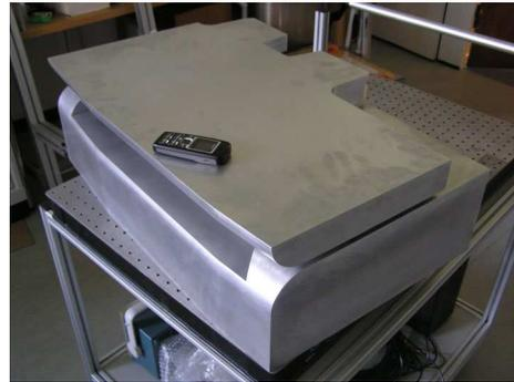
*Fig. 6 1:1 mock-up of the aperture in the vessel wall of ITER*
