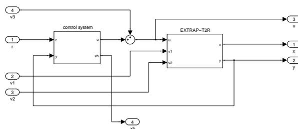
Figure 2: High-level view of SIMULINK setup. Model (1)-(2) feedback-controlled with system (3). Controller objective is to keep a subset of EXTRAP-T2R RWMs at the preset shot reference spectrum  $r(t)$ .
