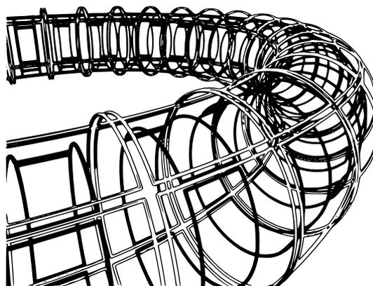
Figure 1: Cartoon of EXTRAP-T2R coil array geometry. Full surface coverage by active saddle coils. Half-width sensor coils inside vessel. Vessel not depicted.
