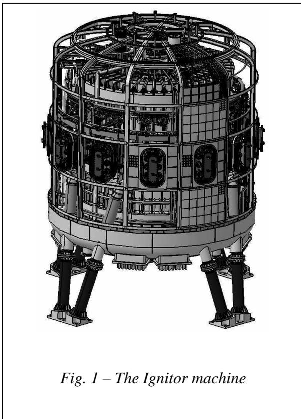
*Fig. 1 – The Ignitor machine*
