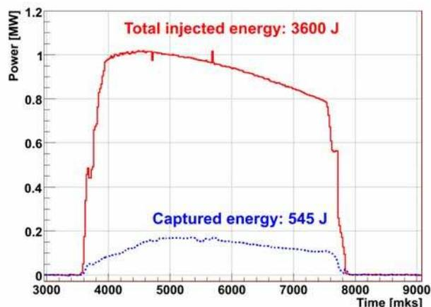
Fig.2 Injected and captured power in the SHIP.
