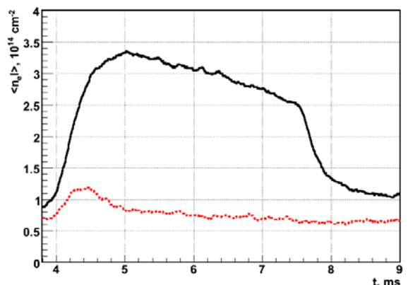
Fig.3 Time evolutions of electron linear density in the SHIP cell during Neutral Beam Injection (solid black line) and without injection (red dotted line).
