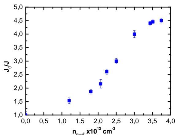
Fig.6 Ion flux suppression vs fast ion density.
