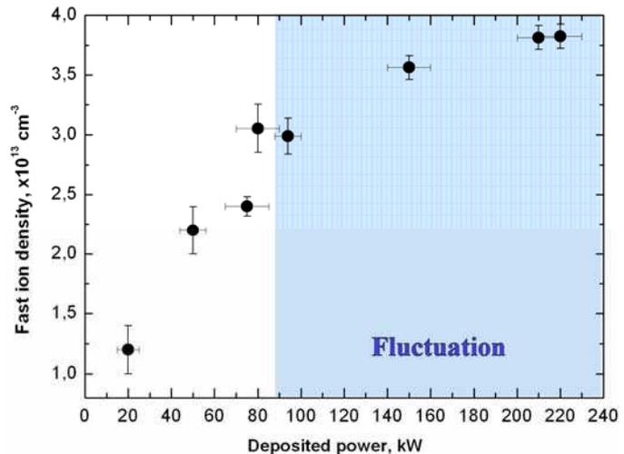
Fig.7 Fast ion density vs. deposited to SHIP NBI power.
