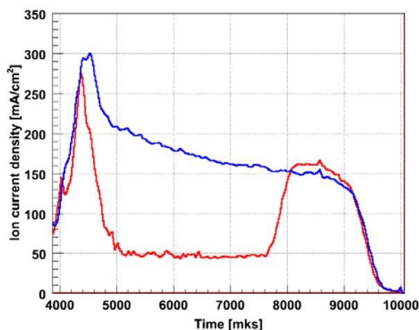
Fig. 5. Time evolutions of ion flux density in the expander cell with NBI in the SHIP cell (red) and without NBI (blue).
