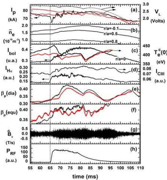
Fig. 1 Basic signals of a discharge with (black line) and without (red line) AW injection. See the text for the definitions.
