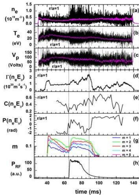
Fig. 2 Triple Langmuir probe signals for a similar discharge to that shown in Fig.1. The probe here was positioned right at the limiter ( $r/a=1$ ). See the text for the definitions
