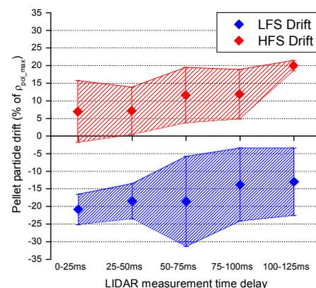
Figure 2 – Average pellet particle drift in JET pellet experiments for LFS and HFS injections and its dependence on the LIDAR measurement delay due to particle transport (diffusion etc.).
