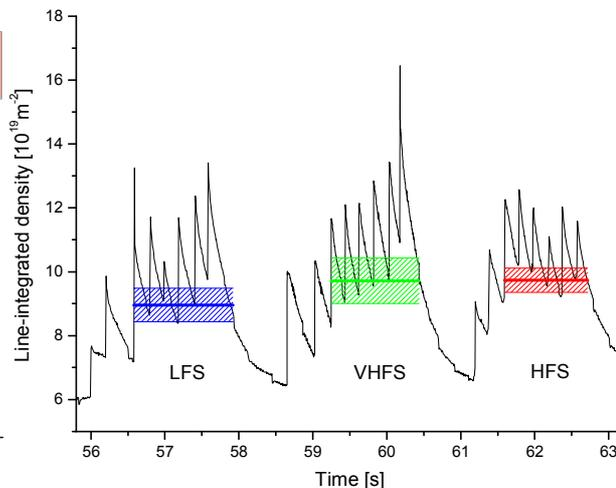
Figure 5 – Time evolution of the line-integrated density signal KG1V/LID3 in the JET experiment #58337, and the density equilibrium level for each pellet injection series (blue: LFS, red: HFS), calculated with the averaged local density minima in the equilibrated phase.
