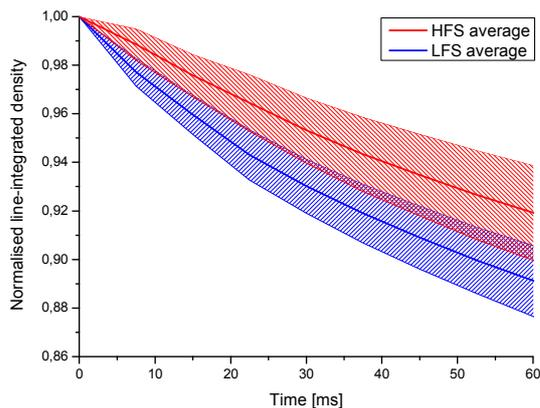
Figure 6 – Averaged normalised line-integrated density decline right after a pellet injection for the LFS and HFS series in the JET experiment #58337. The particles seem to be better retained in the HFS case.
