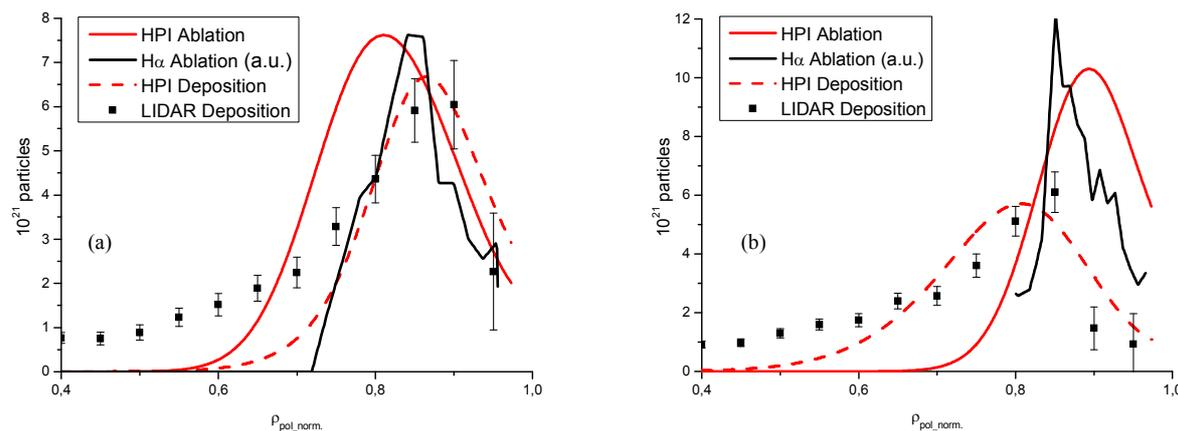
Figure 3 – Comparison of the pellet ablation and deposition profiles, calculated with HPI, with the measurement for two representative pellet injections from the LFS (a) and the HFS (b) in the JET experiment #58337.
