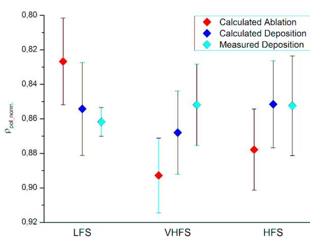
Figure 4 – JET experiment #58337, average calculated particle ablation (red) and deposition (blue) barycentres for each pellet injection direction, compared to the average barycentres of the deposition profiles derived from the interferometer signal (cyan).
