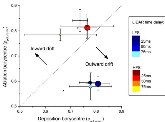
Figure 1 – Average barycentres for the pellet ablation and deposition profiles in the JET pellet database, plotted in dependence of the pellet injection direction and the relative timing of the LIDAR. The size of the circles corresponds to the amount of analysed data. The black squares indicate the position of the average barycentres of the JET exp. #58337.
