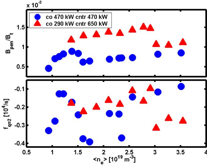
Figure 2: When the excitation threshold suddenly drops at the density of  $1.5 \cdot 10^{19} \text{ m}^{-3}$  (circles) and at  $3 \cdot 10^{19} \text{ m}^{-3}$  (triangles) the toroidal plasma rotation velocity at the  $q=2$  surface also changes to further counter-rotation. No drop is found in the scan with only momentum input in co-direction.
